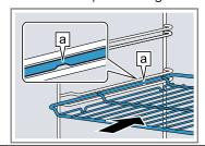
Baking tray E.g. universal pan or baking tray Slide the tray, e.g. the universal pan, in with the sloping edge **b** facing the appliance door.
