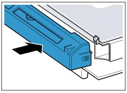
7. Slide the appliance door straight onto the two hinges. Slide the appliance door on as far as it will go. When doing so, ensure that the hinges are inserted into the correct opening.
