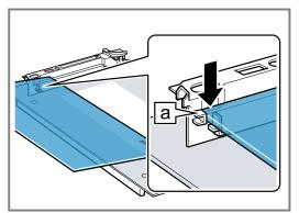
**4.** Slide the inner pane in. In doing so, ensure that the inner pane is in the retainer a.
