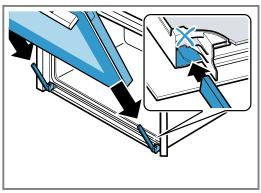
**8.** Close the locking levers on the left- and right-hand hinges.
