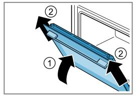
Carefully place the appliance door on a level surface.
