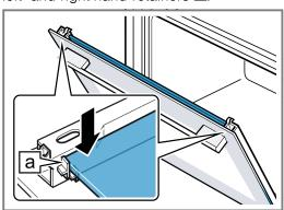
Slide the inner pane into the left- and right-hand retainers a.
