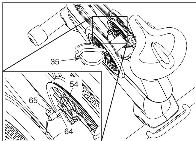
Next, rotate the Left Crank Arm (35) until a Magnet (54) is aligned with the Reed Switch (64). Slide the Reed Switch slightly toward or away from the Magnet. Then, retighten the M4 x 19mm Screw (65).
