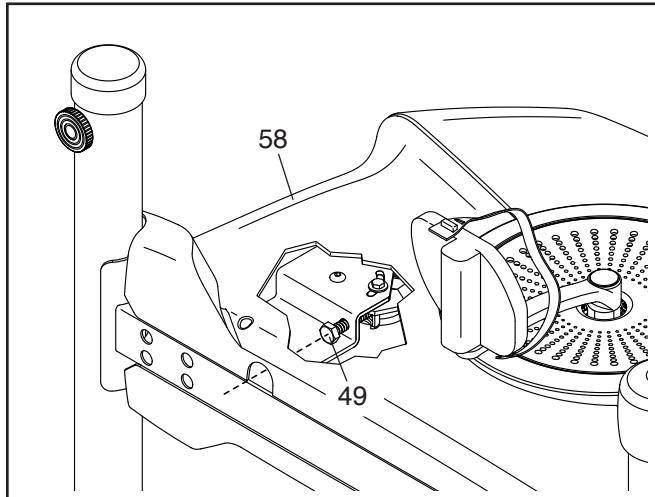
Using an M10 socket wrench with an extension (not included), reach into the opening in the bottom of the Right Shield (58) and tighten the M10 x 50mm Screw (49) a few turns until the Drive Belt (not shown) is tight; **do not overtighten the Drive Belt**.
