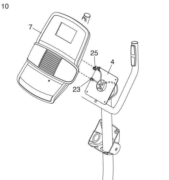
11. **Tip: Avoid pinching the wires.** Attach the Console (7) to the Handlebar (4) with two M4 x 16mm Screws (2) in the lower holes in the Handlebar.
