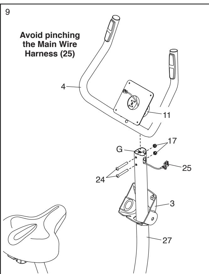
10. Untie and discard the wire tie on the Main Wire Harness (25). Route the Main Wire Harness upward through the Handlebar (4) as shown.
