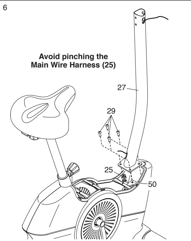
7. Locate the lower end of the wire tie (E) in the Upright (27). Tie the wire tie to the Main Wire Harness (25). Then, pull the upper end of the wire tie until the Main Wire Harness is routed through the Upright and out of the indicated hole (F).
