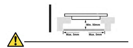
There are ventilation holes around outside of the hob. YOU MUST ensure these holes are not blocked by the worktop when you put the hob into position.
