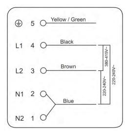
If the total number of heating unit of the appliance you choose is not less than 4, the appliance can be connected directly to the mains by single-phase electric connection, as shown below.
