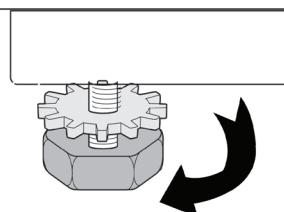
You can adjust the balance of your machine by the adjustable foot.
