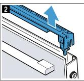
**Note:** Clean the stainless steel inlay in the cover with stainless steel cleaner. Clean the rest of the door cover with soapy water and a soft cloth.
