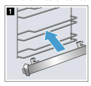
Push the retainer at the back in between the lower and the upper bar (fig. 2).
