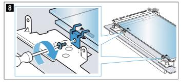
Slide the outer panel back in and make sure that it is sitting correctly at the bottom in the retainer (fig. 9).
