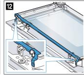
12. Attach the cover and use two screws to secure it (fig. 13).
