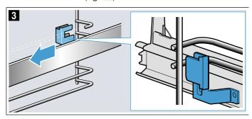
4. Remove the pull-out rail (fig. 4).
