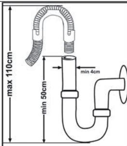
Connect the water drain hose directly to water drain hole or to the sink outlet spigot. This connection should be minimum 50 cm and maximum 110 cm from floor that dishwasher is placed.
