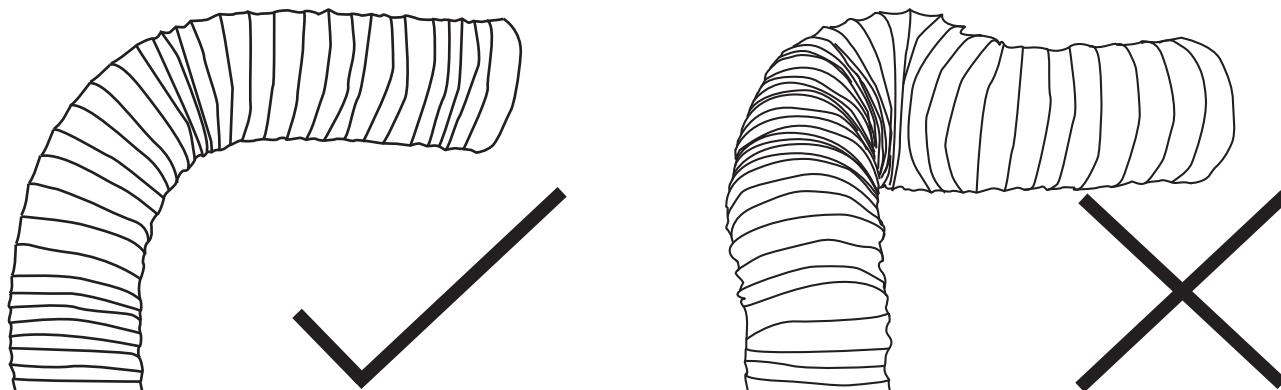
For the Isodrive motors, please do not crush or kink any of the flexi ducting, this will reduce the air flow and may cause noise throughout the system. Ducting needs to be kept taut at all times.
