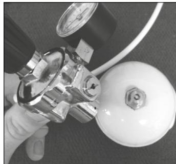
2. Tighten the bottle by rotating anti-clockwise.
