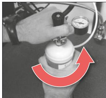
3. Open the pressure regulator by turning the black knob clockwise.
