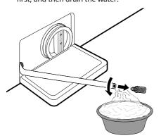
Unscrew the drain pump filter slowly to drain the remaining water and then proceed to remove any debris or objects from the filter.
