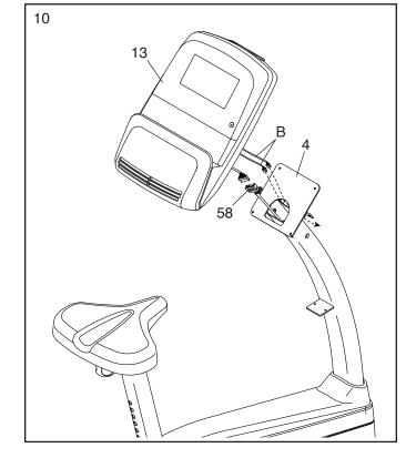
11. **Tip: Avoid pinching the wires.** Attach the Console (13) to the Upright (4) with four #8 x 18mm Screws (34); **start all the Screws, and then tighten them.**
