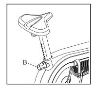
the knob is engaged in one of the adjustment holes in the seat post. Then, tighten the knob.
