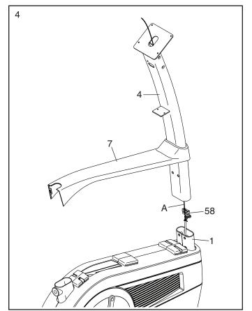
5. **Tip: Avoid pinching the wires.** Slide the Upright (4) onto the Frame (1).
