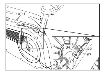
See the lower drawing at the left. Carefully pull the tops of the Shields (10, 11) apart and locate the Reed Switch (57). Rotate the Left Crank Arm (20) until a Magnet (55) is aligned with the Reed Switch. Then, slightly loosen the #8 x 18mm Screw (34), slide the Reed Switch slightly toward or away from the Magnet, and then retighten the Screw.
