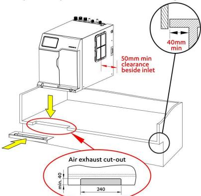
**Option 2. Cupboard with less than 40mm overhang**
