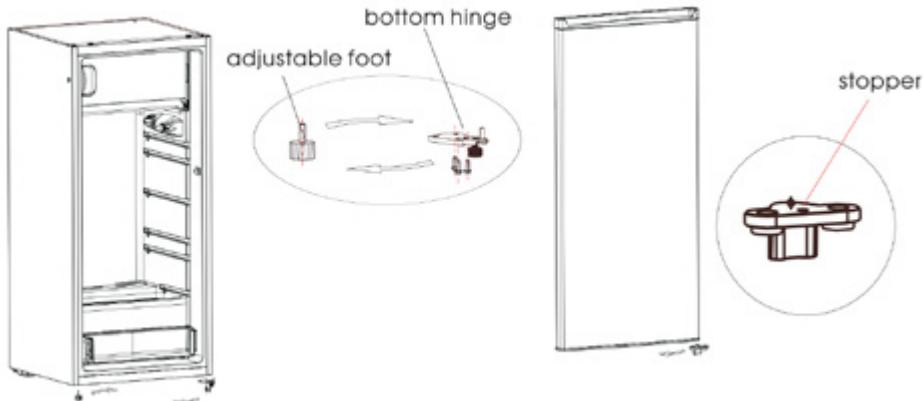
5. Install the door to the bottom hinge, install the upper hinge,upper hinge cover and hole cover on the other side
