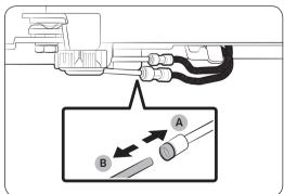
2. To disconnect the hoses, press and hold the transparent coupler (A) and detach the water hose (B).
