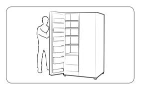
1. Hold the freezer door and hook to the hinge at the bottom of the refrigerator.
