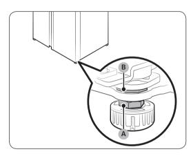
**1.** Open the door to adjust, and locate the two nuts (A) and (B) on the front bottom of the door.
