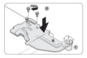
3. Insert the upper hinge shaft (B) into the hinge hole (C). Make sure the hinge shaft is straight so that all screw holes are fully revealed. Then, tighten the hinge screws (D) clockwise.
