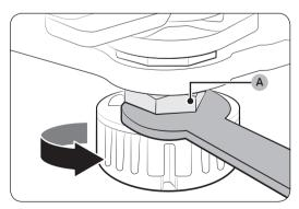
3. When complete, tighten the clamp nut (A) by turning it counter clockwise.
