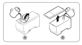
2. Open the front lid (A) of the cover or the entire cover (B) and fill the tank with a max of 5 litres water.
