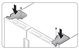
**5.** Insert the hinge covers with the front sides first, and then tighten the screws. Use a Phillips screwdriver for this step.
