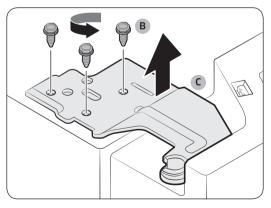
**4.** Unscrew the hinge screws (B) counter clockwise, and remove the upper hinge (C). Be careful as the door can fall on you, causing physical injury.
