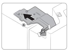
2. On the top side, insert the hinge (A) into the hinge slot.
