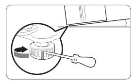
To adjust the height of the freezer side: Insert a flat-head screwdriver into the leveller of the freezer-side front lea. Turn the leveller clockwise to raise, or turn it counter clockwise to lower.
