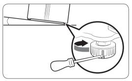
To adjust the height of the fridge side: Insert a flat-head screwdriver into the leveller of the fridge-side front leg. Turn the leveller clockwise to raise, or turn it counter clockwise to lower.
