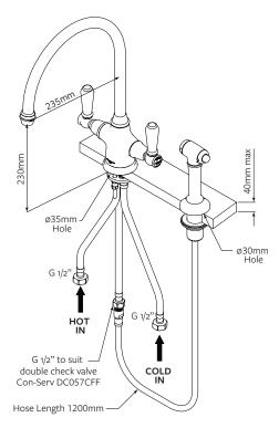
Please Note: This model does not suit incoming water pressure below 100kPa or higher than 500kPa. The spray rinse model requires a minimum inlet pressure of 100kPa to successfully divert the water flow from the main tap to the spray rinse. The stop cocks provided with this tap contain gauze filters. Please ensure your plumber is advised of the minimum and maximum water pressure, and to install the stop cocks as failure to do so voids the tap warranty.
