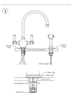
Ensure the mixer is oriented correctly, levers should rotate to point forward and the hot index should be situated on the left. Hot and cold hoses are indicated with a red or blue sticker
