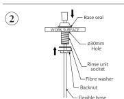
Secure the rinse unit socket in a suitable position using a tap wrench of a 36 AF spanner.
