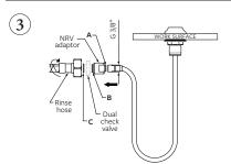
Ensure the black rubber washers are situated inside position A, B (either side of) and C on the rinse hose, including the NRV adaptor in sequence as displayed in the diagram.
