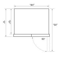
When positioned in a corner area, spacing of at least 285mm on the hinge side will allow the doors to open enough to enable the removal of bins and shelves.
